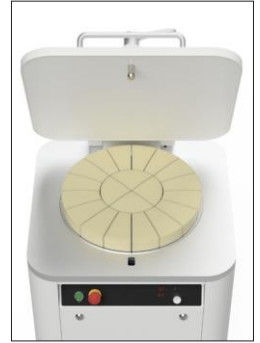
6. Wait for the green button to flash; Open the cover and remove the cut product.
